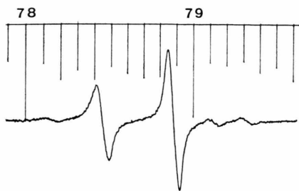
Fig. 3. Central-ion ENDOR spectrum of cubic ZnS:Mn 2+ for \mathbf{H} \parallel [111]_w and T=4.2 K. The spectrum was measured via the -1/2 \leftrightarrow 1/2 ( M_I = -3/2 ) EPR line. The RF power was 5 W, the time-constant 0.3 s and the magnetic field 12.309 KG. The small lines near the main lines are due to forbidden transitions.
